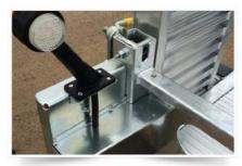
Integrated wiring loom Concealed within chassis affording better protection
